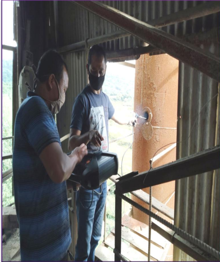
Stack emission monitoring using portable Flue Gas Analyzer at EPIP, Byrnihat
